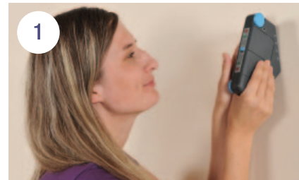
Find the timber studs
