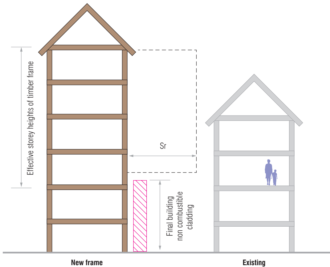
Figure 2.6: Podium and cladding construction options
