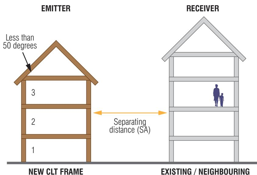
Figure 2 - Separation distance concept in section
