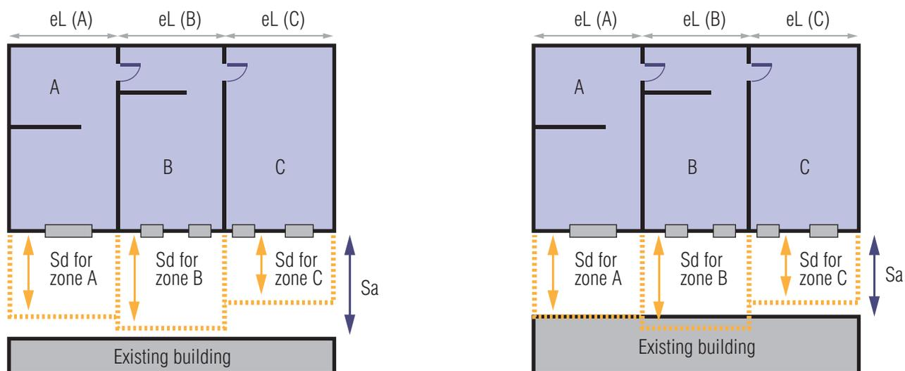
**Figure 8 - Diagrammatic view of checking the safe separation distances from building to building**
