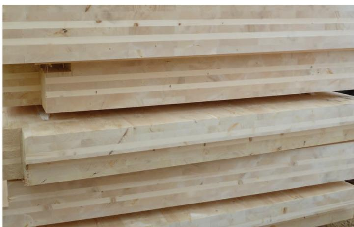
**Image 2 - CLT wall slabs**
