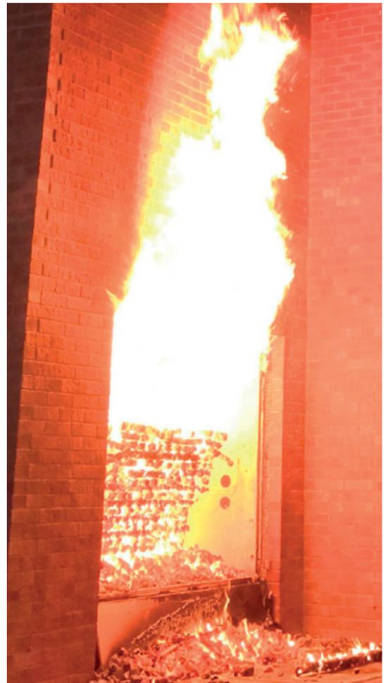
Figure A7.3: Horizontal and vertical fire test for timber batten within the BS8414 test which is a full fire condition of fire from a compartment emitting out of a window
