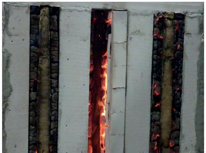
Vertical samples on removal from furnace
