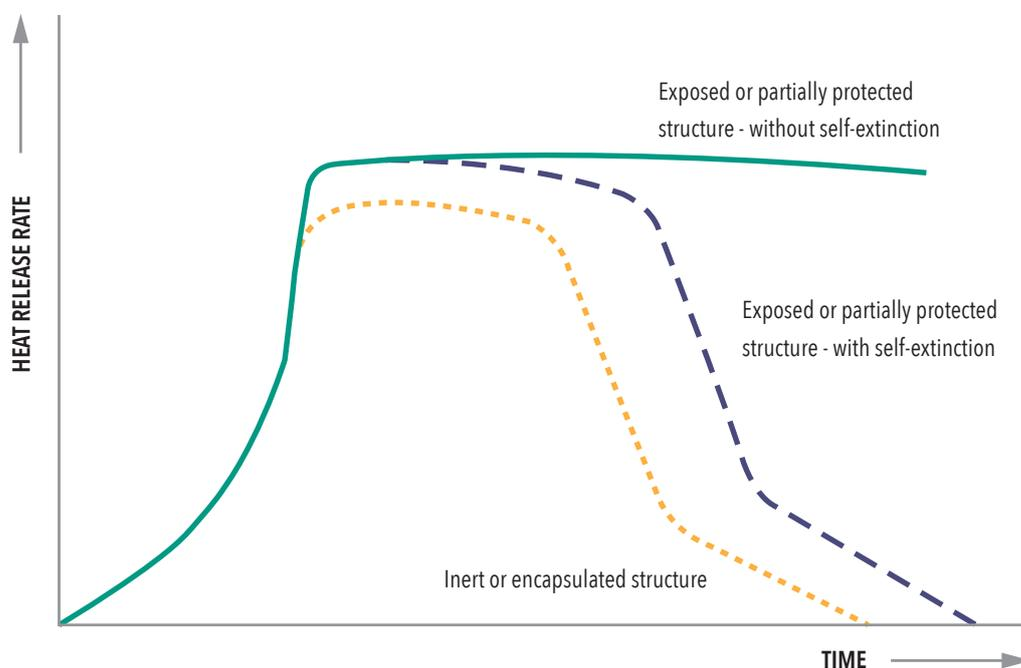
**Figure 1: Conceptual illustration of heat release rate vs. time in inert or combustible enclosures, with or without self-extinction**
