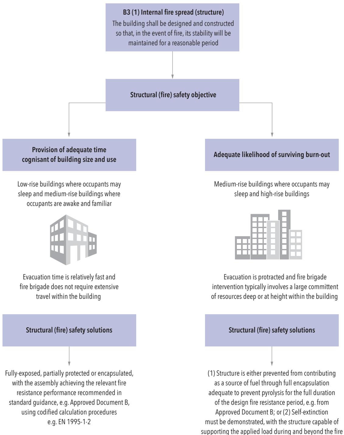
**Figure 3: Illustration of the relationship between structural fire safety objectives, compliance routes and design solutions**
