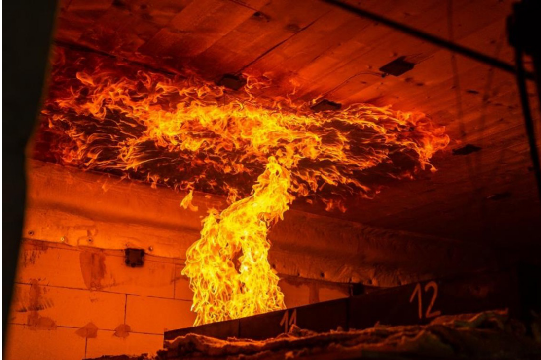
Figure 2: View of the fire enclosure towards the opening with the propane burner shown on the raised plinth
