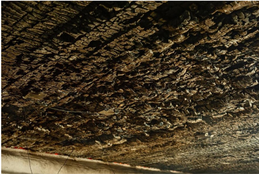
Figure 4: Limited char fall-off above the burner from the CLT with modified PUR adhesive
