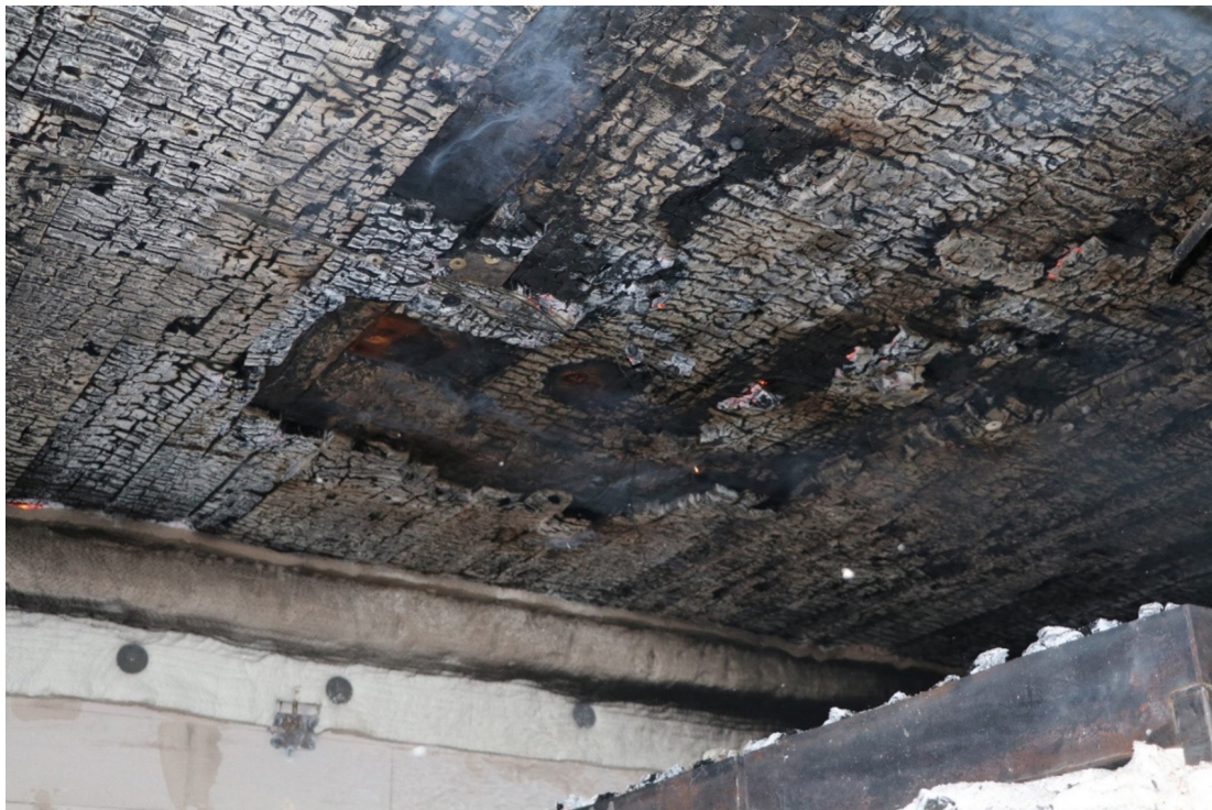
Figure 3: Extensive char fall-off in vicinity of burner from the CLT with the standard PUR adhesive
