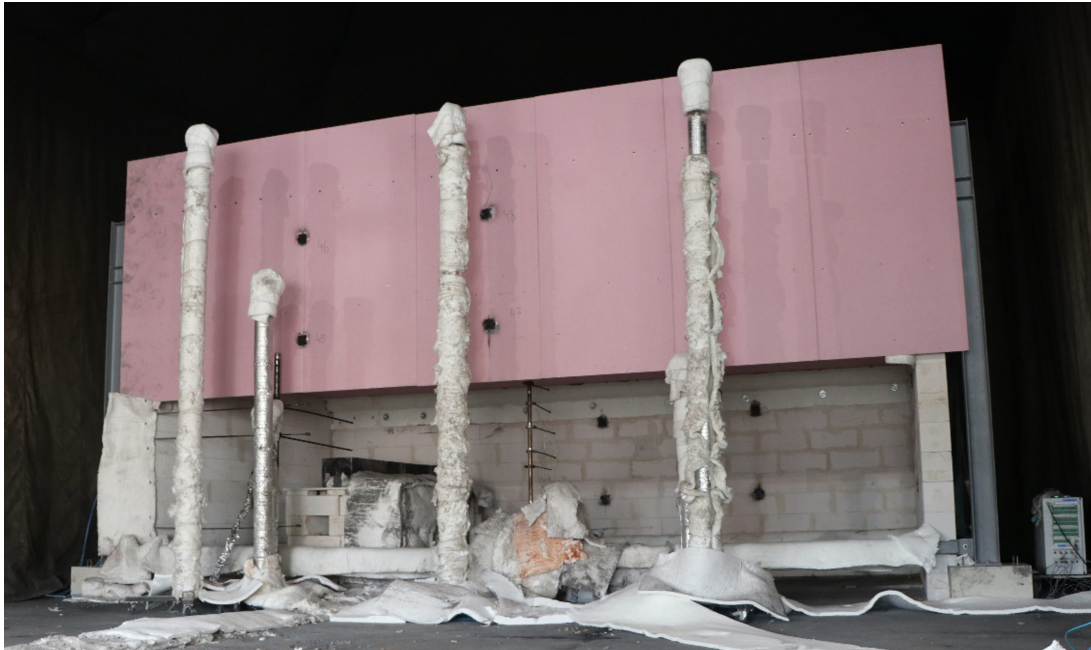
Figure 1: View of the fire enclosure towards the opening with the propane burner shown on the raised plinth
